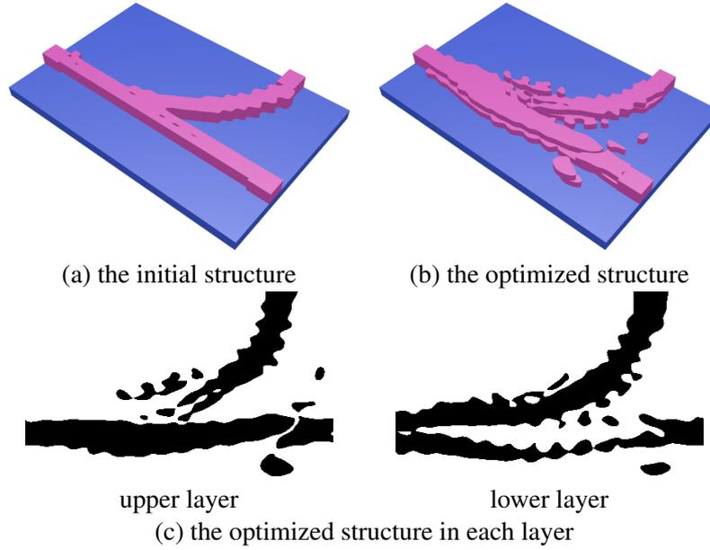
Figure 2: Topology optimized PSR with two layers.
