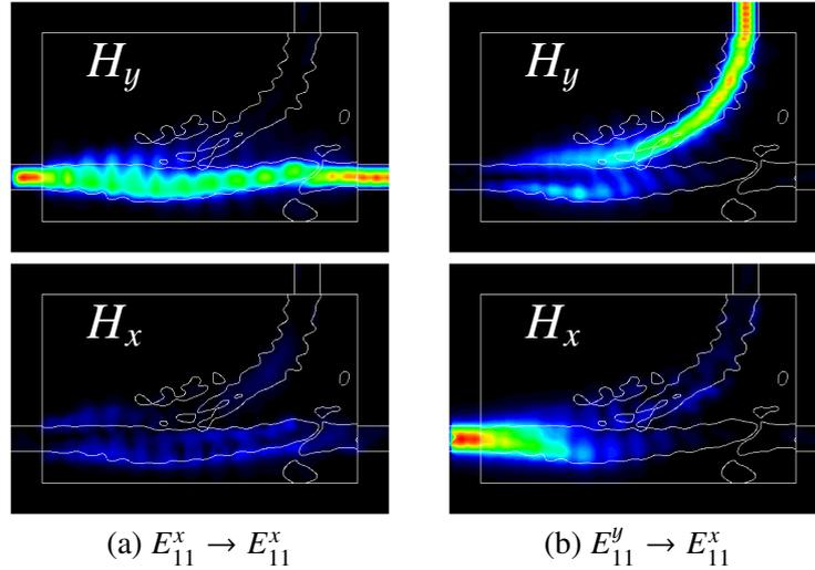
Figure 3: Propagating field in the optimized PSR.
