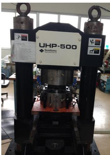
Fig 2.2.1 A cubic anvil high-pressure apparatus (Sumitomo Heavy Industries UHP-500), Muroran Institute of technology.
