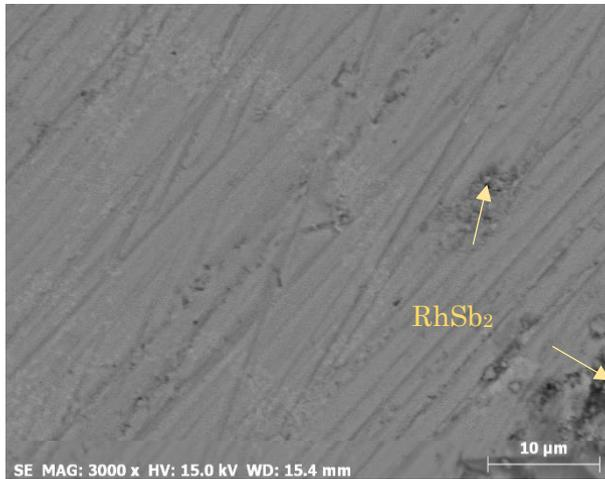
SEM image #5:  $\text{Yb}_{0.6}\text{Rh}_4\text{Sb}_{12}$
