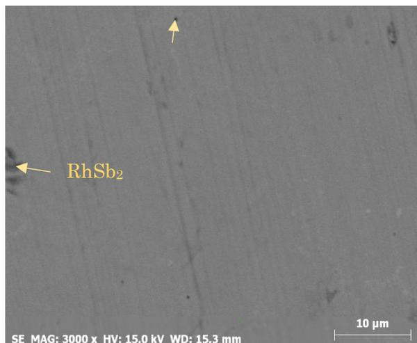
SEM image #3:  $\text{Yb}_{0.4}\text{Rh}_4\text{Sb}_{12}$
