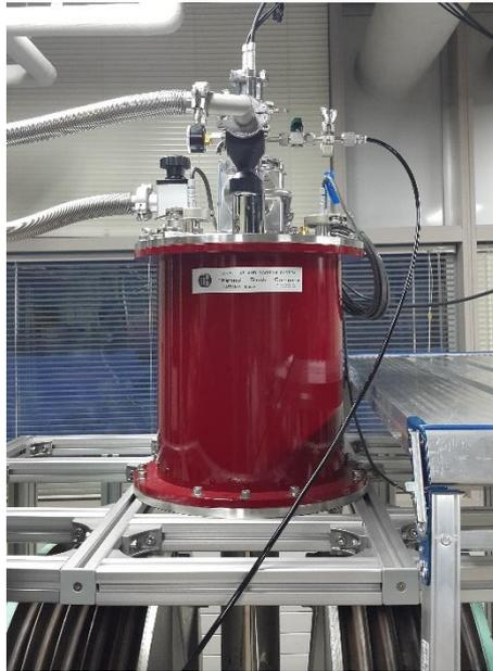
Fig 2.4.3. A cryostat and vacuum system (Thermal block company, Saitama Japan), Muroran Institute of technology, Hokkaido, Japan
