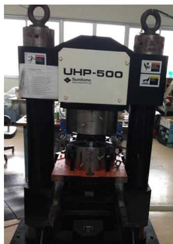
Fig 1.4.1 a cubic anvil apparatuses of UHP-500
