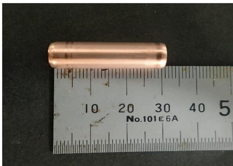
**Figure 2.1** The copper deoxidized phosphor tube specimen
