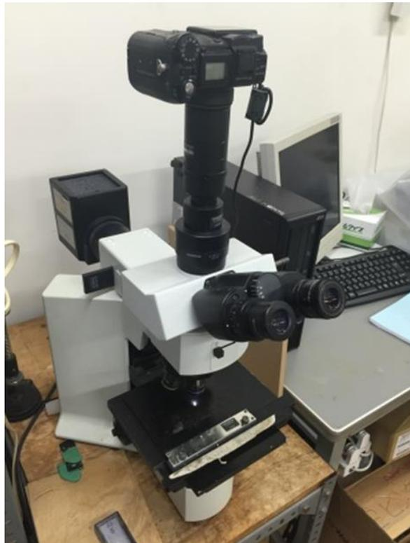
Figure 2.6 Microscope BX51M.
