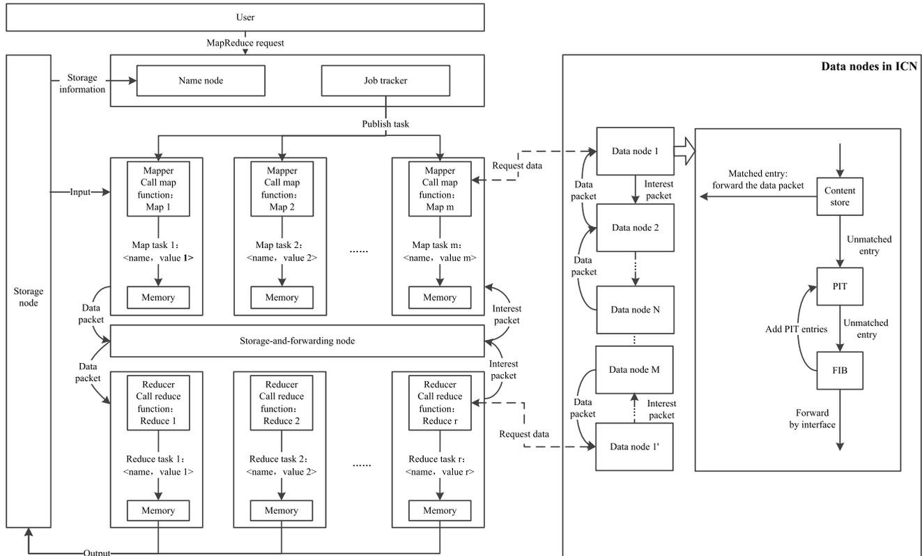
FIGURE 3. MapReduce-ICN architecture specific network [37].
