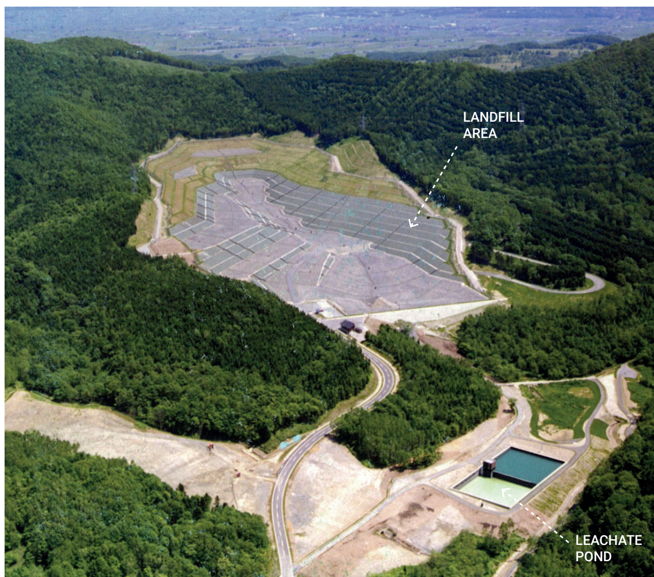
FIGURE 1: Aerial view of the operating semi-aerobic landfill in the northern part of Hokkaido, Japan (in 2003).
