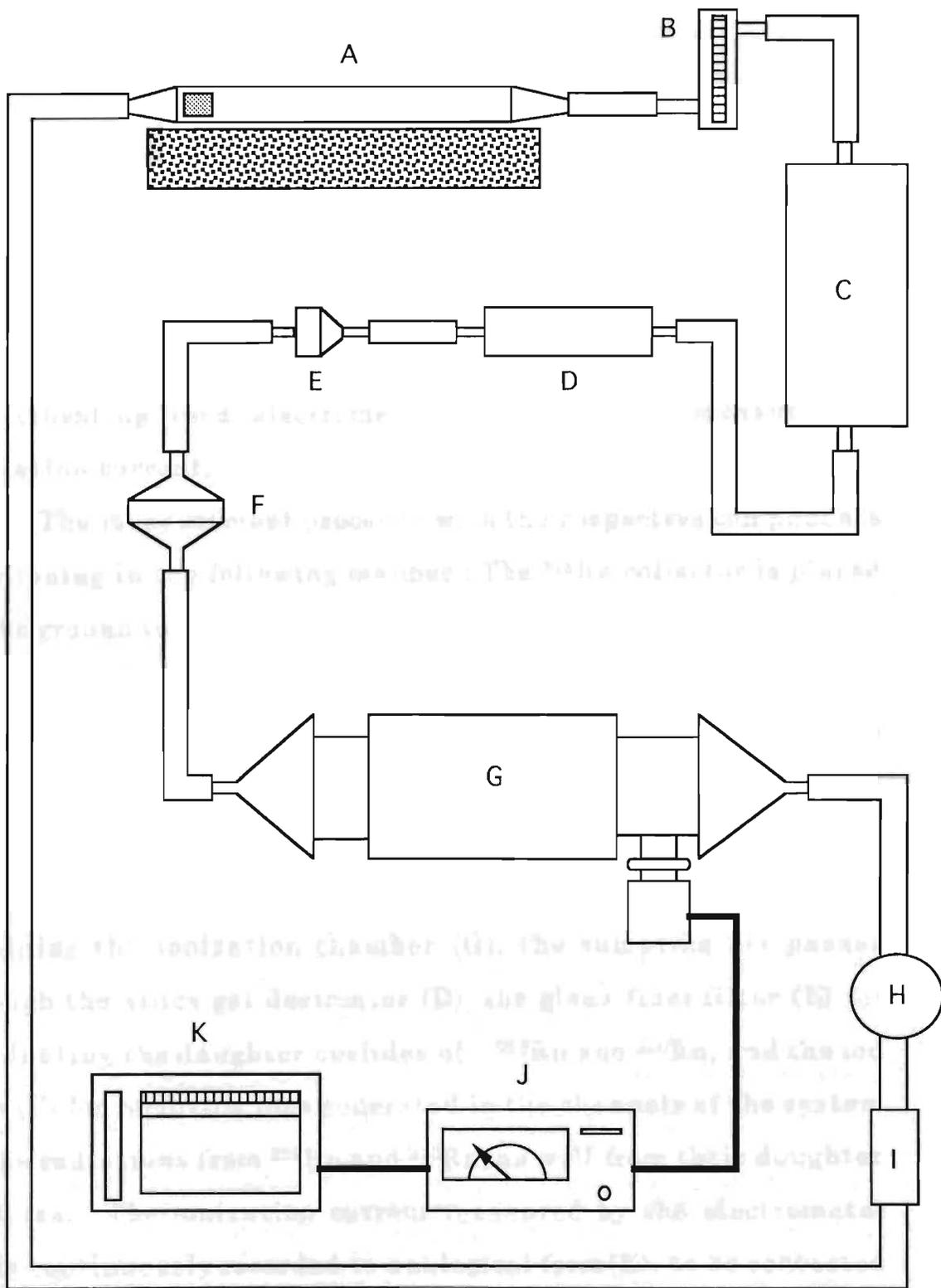
Fig. 2-2 Arrangement of apparatus for measuring ionization current generated by  $^{222}\text{Rn}$  exhalation from ground.
