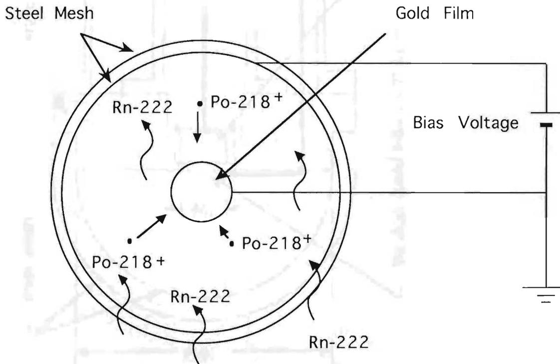
Fig. 1-1 Schematic representation of the measuring principle.
