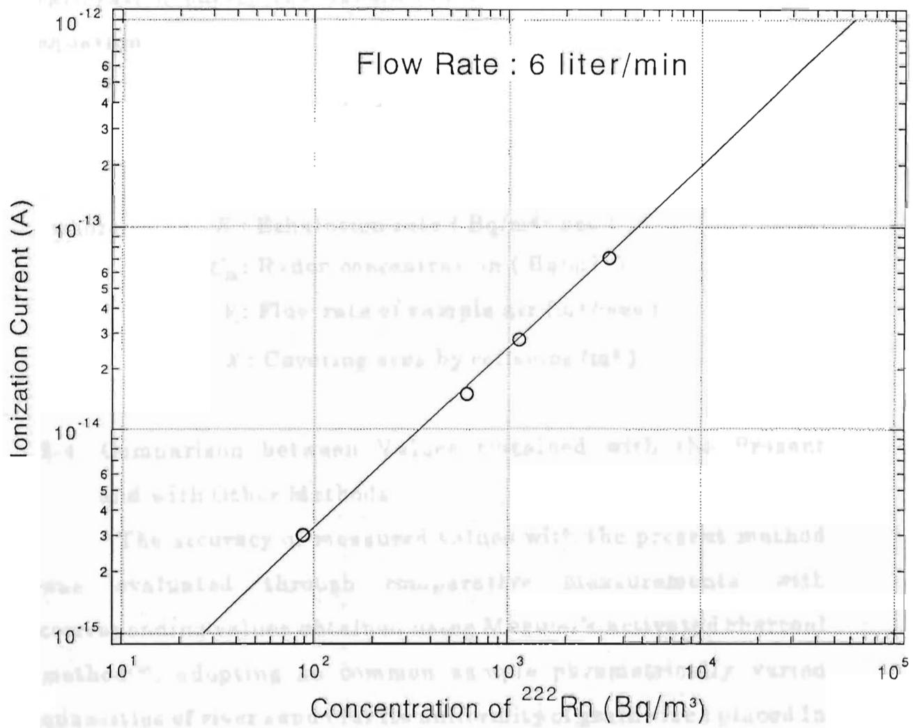
Fig. 2-3 Calibration plots relating measured ionization current to  $^{222}\text{Rn}$  concentration
