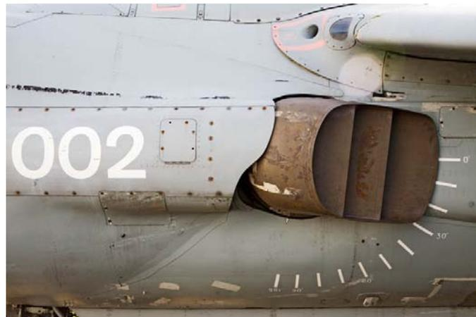
Figure 1.1 Sea Harrier FA.2 ZA195 front (cold) vector thrust nozzle.
