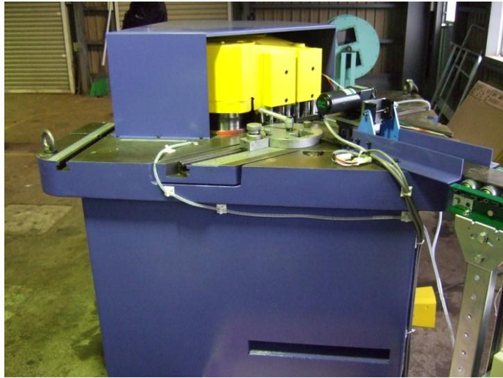
Fig. 5-4 Photos of guillotine cutting testing machine.
