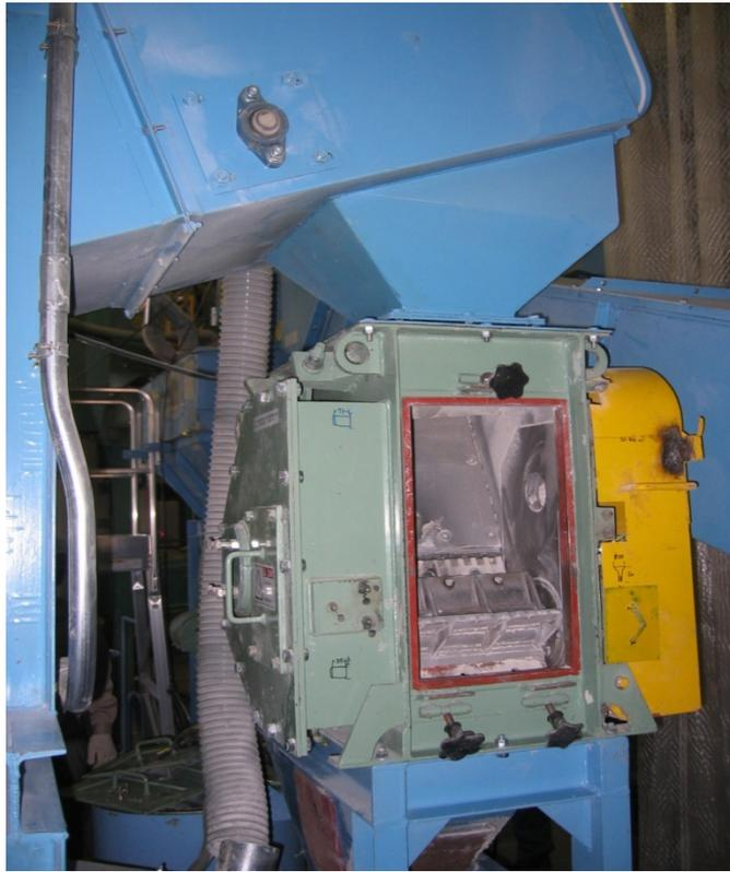
Fig. 4-3 Uniaxial rotational glass shredder.
