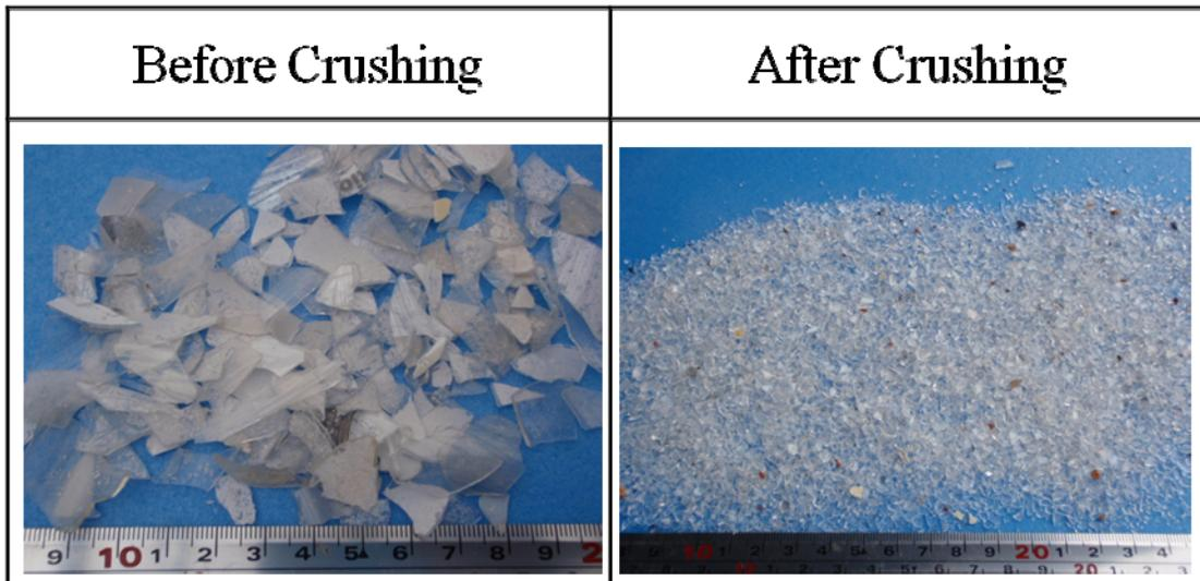
Fig. 4-4 Crushed glass of waste fluorescent lamp.
