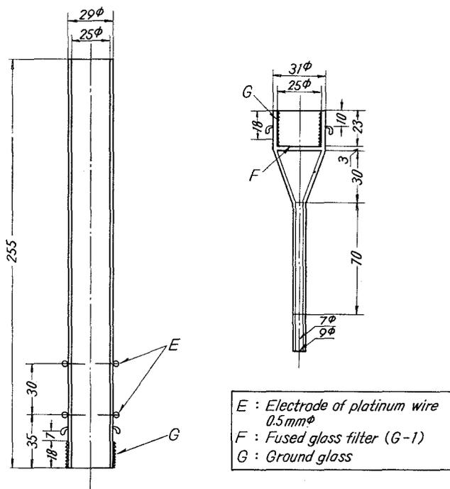
Fig. 2. Details of combustion chamber made of hardglass.
