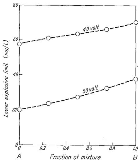
Fig. 9. Lower explosive limit of dust mixture of wood charcoal A and B
