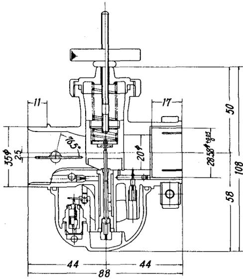
Fig.2 Test carburettor (Engine E-120)
