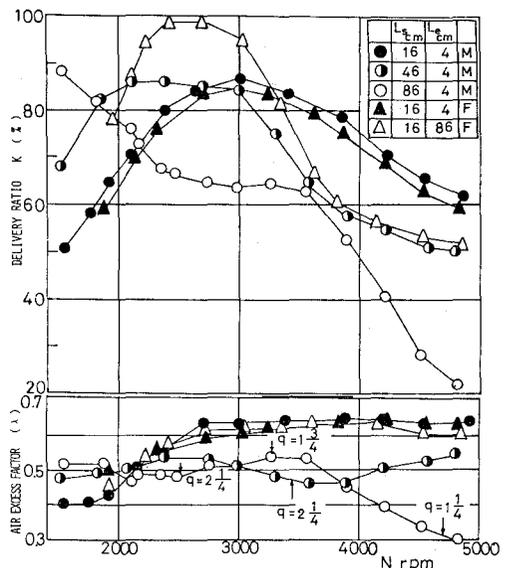
Fig.11 Delivery ratio  $K$ , excess air ratio  $\lambda$  and engine speed  $N$  (Engine E-120)
