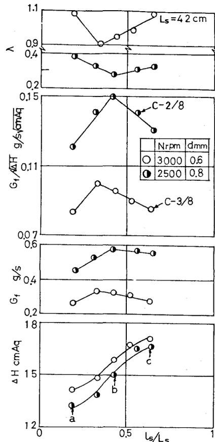
Fig.19 Excess air ratio  $\lambda$  and carburettor position  $l_s/L_s$  (Engine E-120)
