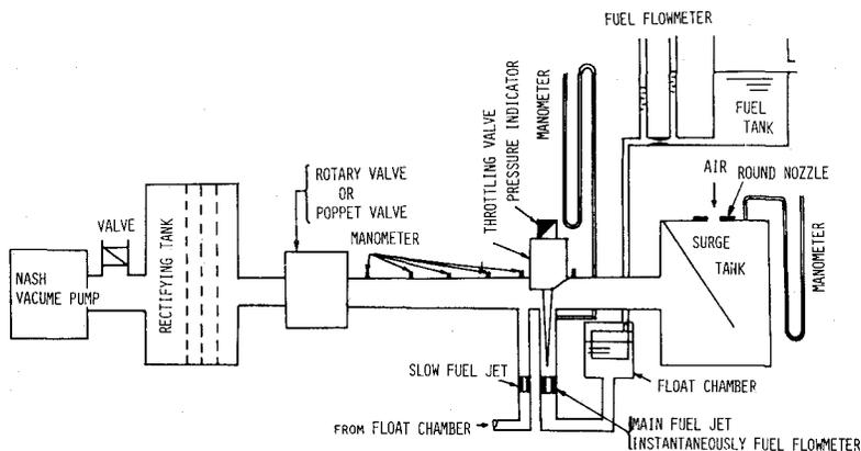
Fig.1 General layout of testing apparatus (carburettor experiment)
