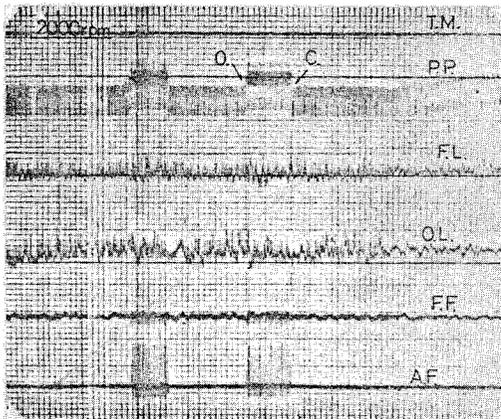
**Fig.25** Behavior of float (F.L.) and fuel level (O. L.)
