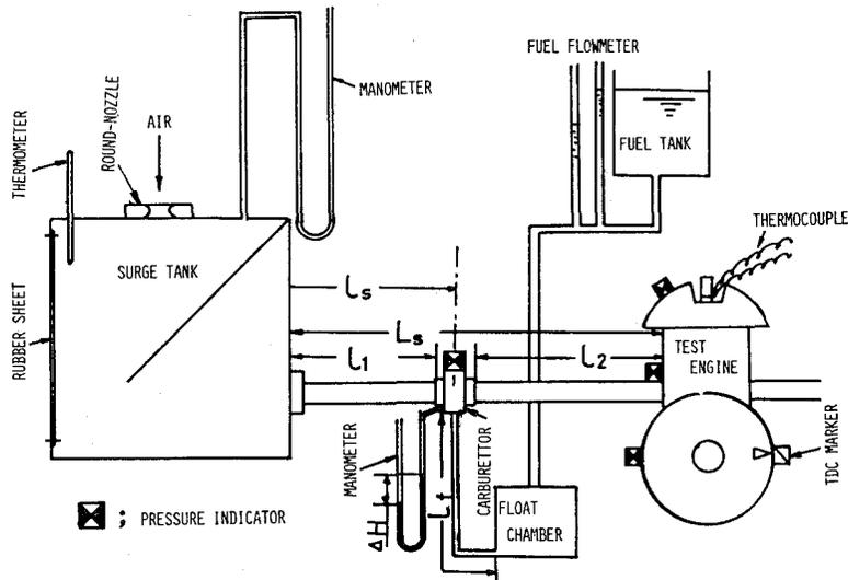
Fig.6 General layout of testing apparatus (engine experiment)
