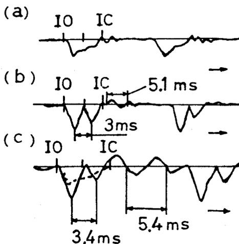
Fig.20 Fluctuating pressure in carburettor throat
