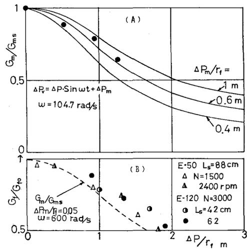
Fig.14 Ratio of fuel flow rate  $G_m/G_{ms}$ ,  $G_f/G_{fo}$  and pulsating pressure wave
