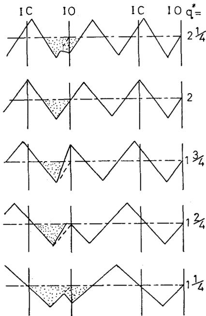
Fig.10 Pulsation factor  $q^*$  and superpose of pressure wave
