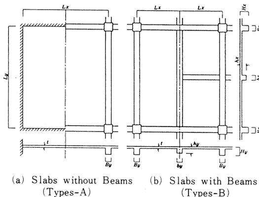
(a) Slabs without Beams (Types-A) (b) Slabs with Beams (Types-B)
