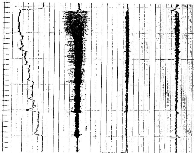
Fig. 14 Force-curve and EMG at contraction with increasing load in subj. K.T.
