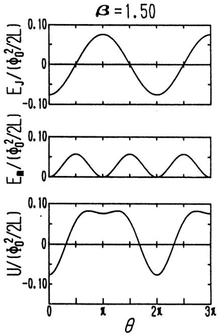
Fig. 21  $E_J$ ,  $E_m$  and system energy  $U$  as a function of  $\theta$  for  $\beta = 1.50$ .
