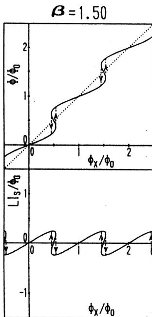
**Fig. 27** Internal flux  $\Phi$  and the induced flux  $LI_s$  as a function of  $\Phi_x$  for  $\beta = 1.50$ . The hysteresis with transitions at different  $\Phi_x$  is indicated by arrows. The hysteresis behavior corresponds to that in Fig. 9.
