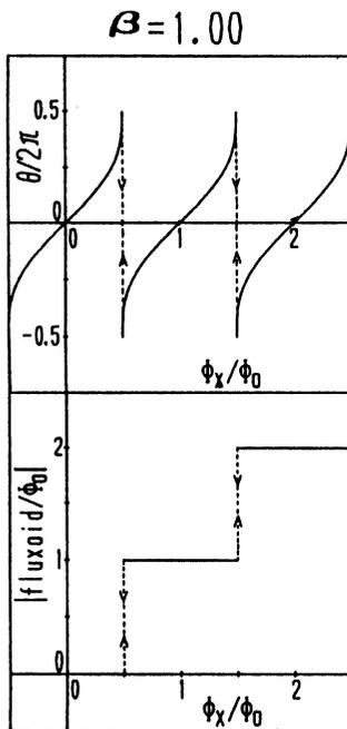
Fig. 32 Phase difference  $\theta$  and fluxoid as a function of  $\Phi_x$  for  $\beta = 1.00$ .
