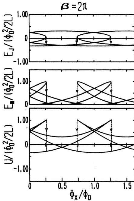
Fig. 17  $E_J$ ,  $E_m$  and  $U$  as a function of  $\Phi_x$  for  $\beta = 2\pi$ . The hysteresis behavior can be understood by considering the correspondence between Fig. 11 and Fig. 17. The value of  $U$  corresponds to the minimum or maximum value in Fig. 11.
