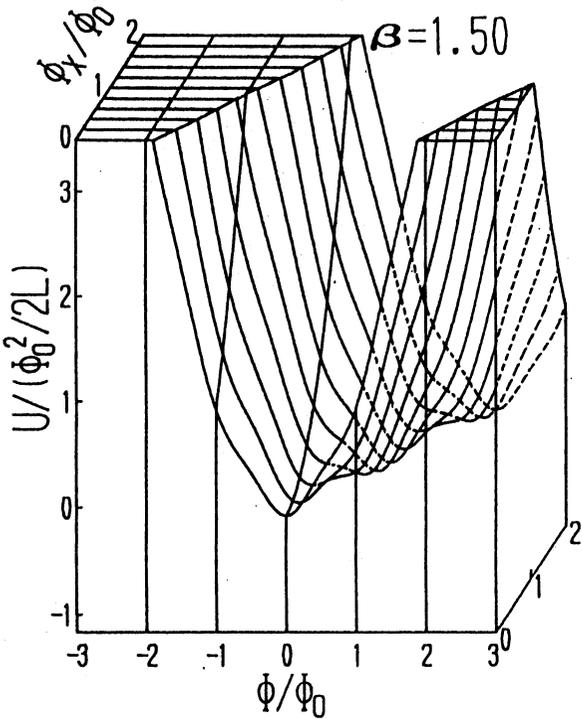
**Fig. 4** Potential  $U(\Phi, \Phi_x)$  surface for  $\Phi_x = 0$  to  $2\Phi_0$  and  $\Phi = 3\Phi_0$  to  $-3\Phi_0$  in the case where  $\beta = 1.50$ . The sharp transitions can occur between the two adjacent quantum states at  $\Phi_x = 0.544\Phi_0$  and  $0.456\Phi_0$  in the irreversible process, see Fig. 9.
