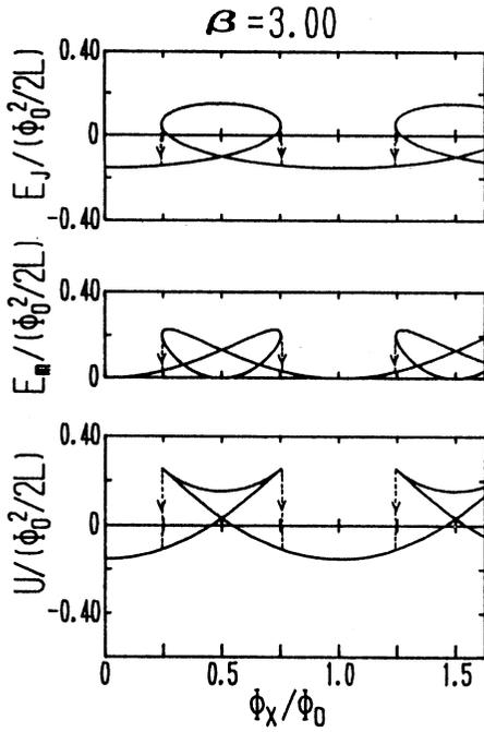
Fig. 16  $E_J$ ,  $E_m$  and  $U$  as a function of  $\Phi_x$  for  $\beta = 3.00$ . The hysteresis behavior can be understood by considering the correspondence between Fig. 10 and Fig. 16. The value of  $U$  corresponds to the minimum or maximum value in Fig. 10.
