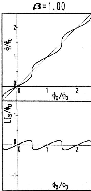
**Fig. 26** Internal flux  $\Phi$  and the induced flux  $LI_s$  as a function of  $\Phi_x$  for  $\beta = 1.00$ .
