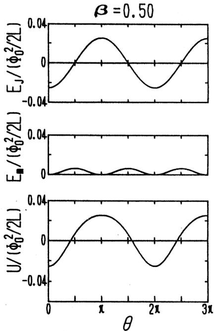
Fig. 19  $E_J$ ,  $E_m$  and system energy  $U$  as a function of  $\theta$  for  $\beta = 0.50$ .
