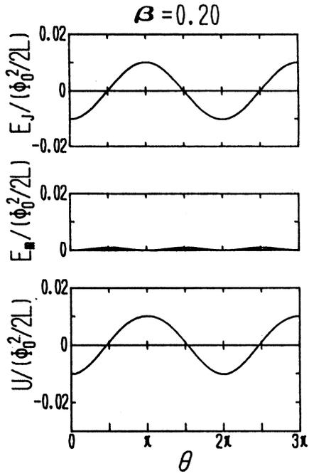
Fig. 18 Junction coupling energy  $E_J$ , magnetic energy  $E_m$  and system energy  $U$  as a function of the phase difference  $\theta$  across the junction for  $\beta = 0.20$ .
