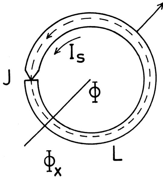
**Fig. 1** Superconducting ring with a ideal Josephson junction denoted by  $J$ . The contour used for integration is shown by the broken line. Internal magnetic flux  $\Phi$ , circulating current  $I_s$ , self - inductance  $L$  and applied magnetic flux  $\Phi_x$  are related by  $\Phi = \Phi_x - LI_s$ . Typical values are  $L = 5$  nH, and  $I_0 = 1 \mu$  A. The junction resistance in the normal state is  $R = 10 \Omega$ , and the diameter of the ring is about 2mm.
