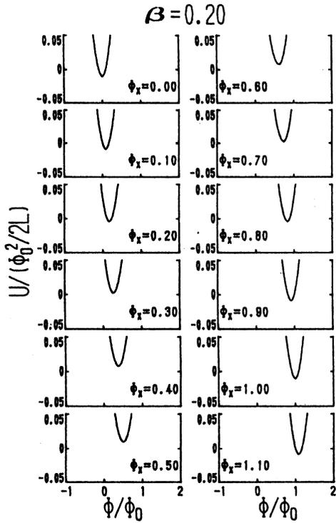
**Fig. 6** System energy  $U$  for  $\beta = 0.20$  as a function of  $\Phi$ . The energy minimum shifts gradually from a flux quantum state to a neighbor state when the external magnetic flux  $\Phi_x$  changes. The value of  $\Phi_x$  denoted in each graph is normalized by  $\Phi_0$ .
