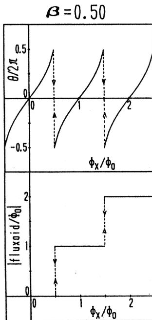
**Fig. 31** Phase difference  $\theta$  and fluxoid as a function of  $\Phi_x$  for  $\beta = 0.50$ .
