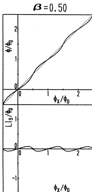
Fig. 25 Internal flux  $\Phi$  and the induced flux  $LI_s$  as a function of  $\Phi_x$  for  $\beta = 0.50$ .
