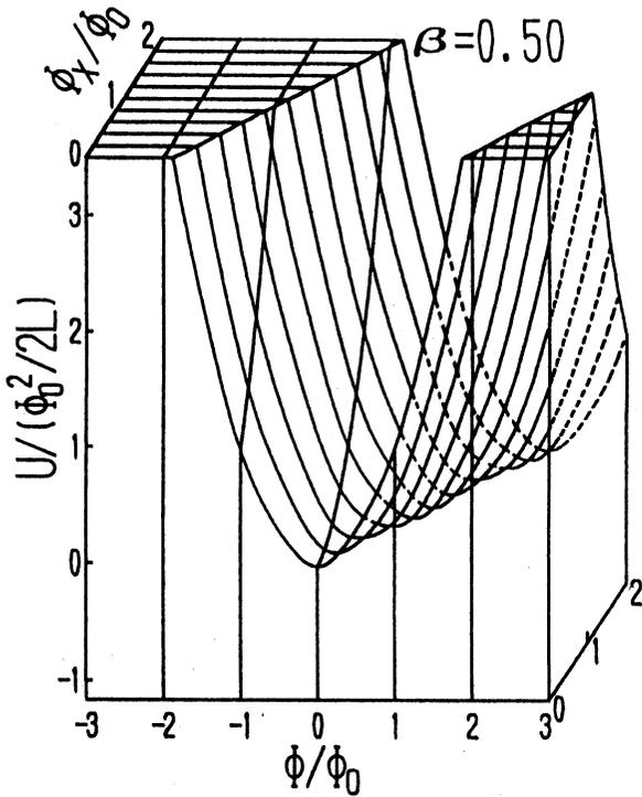
**Fig. 3** Potential  $U(\Phi, \Phi_x)$  surface for  $\Phi_x = 0$  to  $2\Phi_0$  and  $\Phi = 3\Phi_0$  to  $-3\Phi_0$  in the case where  $\beta = 0.50$ . The sharp transition can not occur between the two adjacent quantum states.
