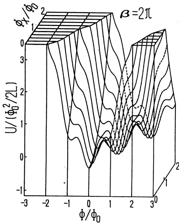
**Fig. 5** Potential  $U(\Phi, \Phi_x)$  surface for  $\Phi_x = 0$  to  $2\Phi_0$  and  $\Phi = 3\Phi_0$  to  $-3\Phi_0$  in the case where  $\beta = 2\pi$ . The sharp transitions can occur between the two adjacent quantum states, see Fig. 11.
