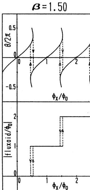
Fig. 33 Phase difference  $\theta$  and fluxoid as a function of  $\Phi_x$  for  $\beta = 1.50$ . The hysteresis with transitions at different  $\Phi_x$  is indicated by arrows. The hysteresis feature corresponds to that in Fig. 9.
