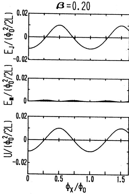
Fig. 12 Junction coupling energy  $E_J$ , magnetic energy  $E_m$  and system energy  $U$  as a function of the external flux  $\Phi_x$  for  $\beta = 0.20$ . The value of  $U$  corresponds to the minimum value in Fig. 6.
