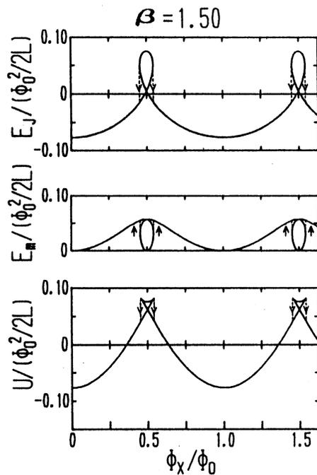
Fig. 15  $E_J$ ,  $E_m$  and  $U$  as a function of  $\Phi_x$  for  $\beta = 1.50$ . The hysteresis with transitions at different  $\Phi_x$  is indicated by arrows. The hysteresis behavior can be understood by considering the correspondence between Fig. 9 and Fig. 15. The value of  $U$  corresponds to the minimum or maximum value in Fig. 9.
