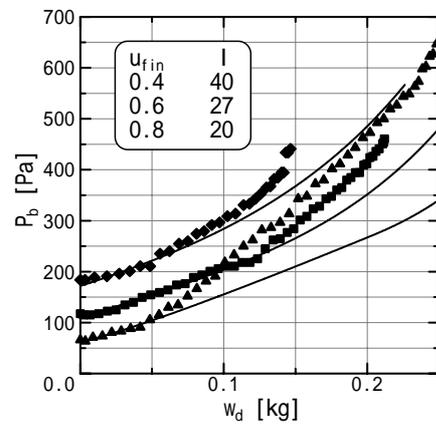
Fig.11 Theoretical collection efficiency and pressure drop in small scale fixed bed ring filter
