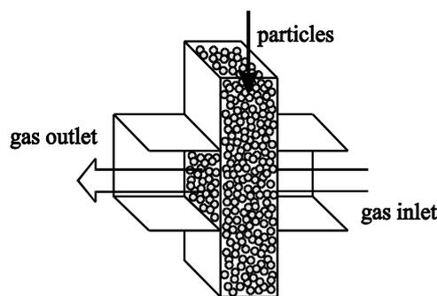
Fig.1 Parallel panel filter
