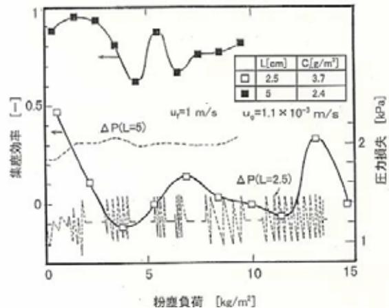
Fig.4 Changes of collection efficiency and pressure drop with dust loading
