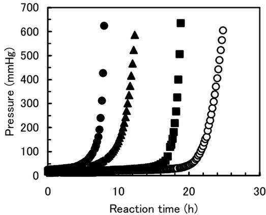
Fig. 12 Effect of hardness material addition on hydrogen evolution by mechano-chemical reaction of aluminum with water. (○) no addition, (●) BN (4 g), (▲) SiC (8 g), (■) SiO<sub>2</sub> (6 g).
