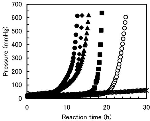
Fig. 7 Effect of addition of various hardness materials (6.0 g) on hydrogen evolution by mechano-chemical reaction of aluminum with water. (○) no addition, (●) SiC, (◆) Cr, (▲) BN, (■) SiO<sub>2</sub>, (×) WC.
