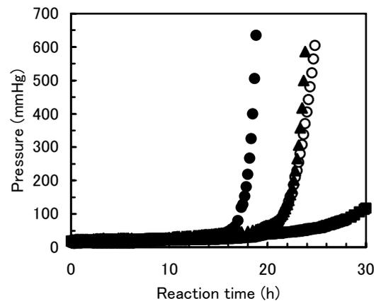
Fig. 10 Effect of the amount of SiO<sub>2</sub> addition on hydrogen evolution by mechano-chemical reaction of aluminum with water. (○) 0 g, (▲) 3 g, (●) 6 g, (■) 8 g.
