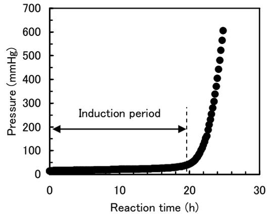
Fig. 3 Hydrogen evolution by mechano-chemical reaction of aluminum and water.
