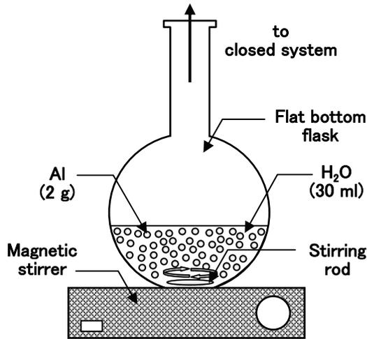
Fig. 1 Reactor for mechano-chemical reaction of aluminum with water.
