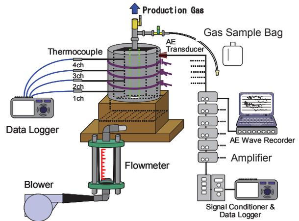
Fig. 2. Experimental setup for coal block specimen
