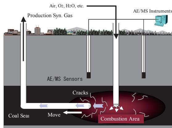
Fig. 1. UCG system and AE/MS monitoring system
