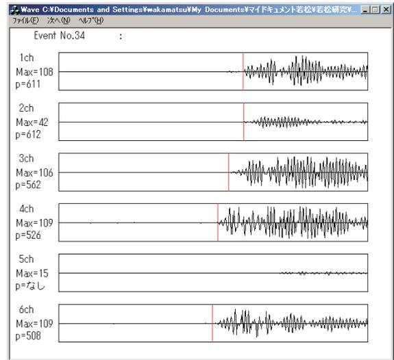
Fig. 5. Typical AE waveforms for source locations
