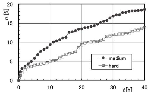
Fig. 11 Effect of bristle stiffness on removal area ratio  $\alpha$  for rubbing time  $t$  ( $v = 52.4$  mm/s,  $W = 3.52$  N, SUS)
