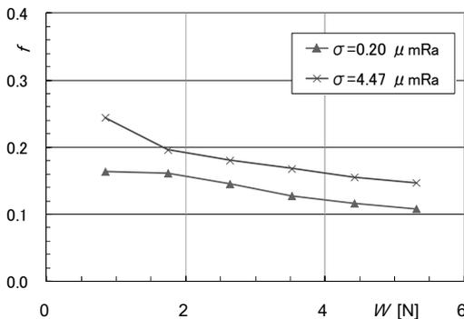
Fig. 8 Effect of roughness on friction coefficient  $f$  ( $v = 52.4$  mm/s, PTFE, medium, dry)
