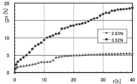
Fig. 9 Effect of load on removal area ratio  $\alpha$  for rubbing time  $t$  ( $v = 52.4$  mm/s, SUS, medium)
