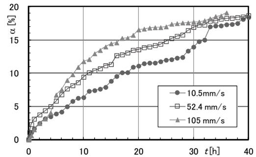
Fig. 10 Effect of speed on removal area ratio  $\alpha$  for rubbing time  $t$  ( $W = 3.52$  N, SUS, medium)
