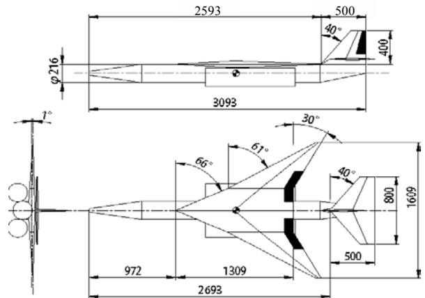
図2. M2006prototype 形状
