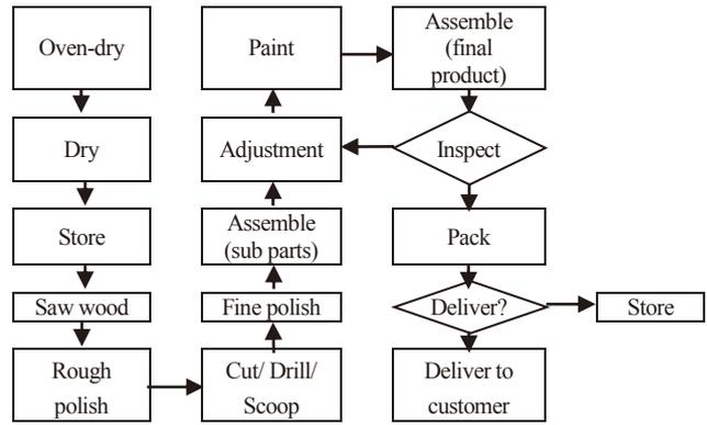
Figure 4 Production process at the case study company
