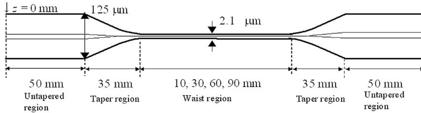
Fig. 2 Schematic structure of a biconical tapered fiber.
