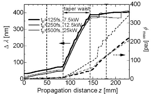
Fig. 8 Evolution of the spectral width  $\Delta\lambda$  and maximum phase value  $\phi_{\max}$  as a function of the propagation distance  $z$  for  $t_p=125$  fs,  $P_p=7.5$  kW and  $t_p=250$  fs,  $P_p=12.5$  kW and  $t_p=500$  fs,  $P_p=25$  kW with waist length  $L_w=60$  mm.
