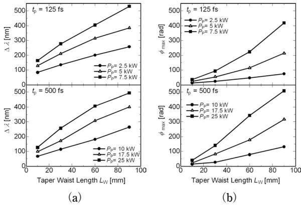
Fig. 9 (a) SC spectral width  $\Delta\lambda$  and (b) maximum phase value  $\phi_{\max}$  as a function of waist length  $L_W$  of different peak powers  $P_P$  for pulse widths of 125 fs and 500 fs.
