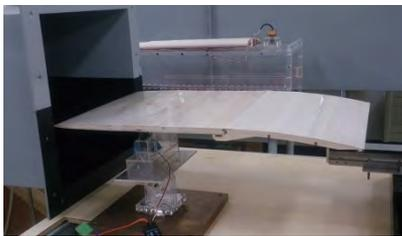
Fig. 5. A flat plate wing with a parabolic rear surface.
