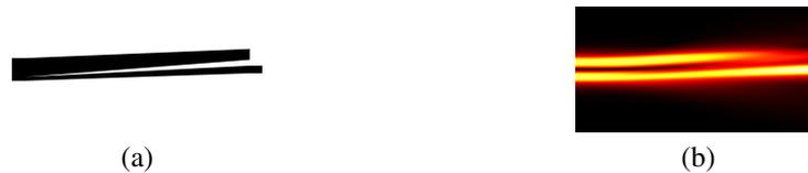
Fig. 14. Optimized structure of a  $TE_0$ -to- $TE_1$  converter based on an asymmetric branching waveguide and propagation wave.
