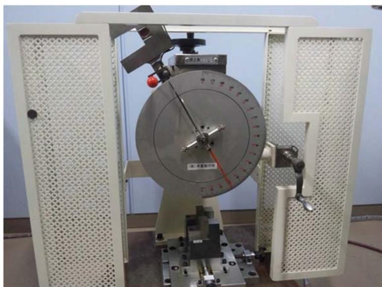
Fig.5-4 Machine for impact test
