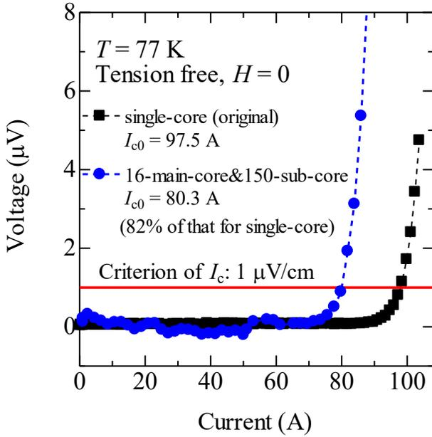
Fig. 3. Current-voltage curves for original coated conductor and 16-main-core split wire in tension-free state without an external magnetic field. The criterion for the critical current  $I_c$  was  $1 \mu$ V/cm.
