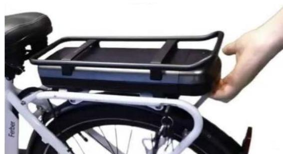
(d) The installation and removal of the battery are less than 10 seconds
