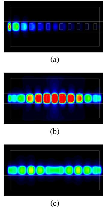
Fig. 9. Magnetic field distribution obtained by FEM analysis corresponding to the problem shown in Fig.6: (a) $\lambda = 1.55$   $\mu\text{m}$ ; (b) $\lambda = 1.632$   $\mu\text{m}$ ; (c)  $\lambda = 1.85$   $\mu\text{m}$ .
