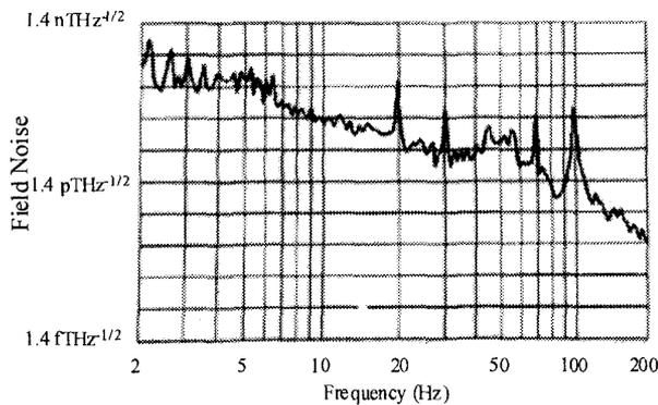
Fig. 2. A magnetic flux noise spectrum measured with High Tc SQUID.
