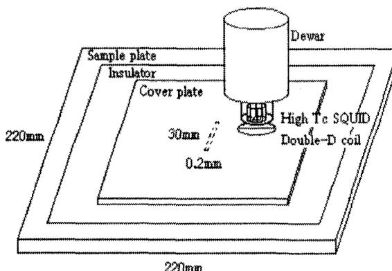
Fig. 1. The geometry of the scanning system.
