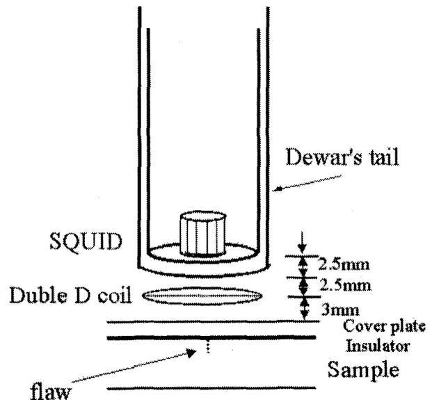
Fig. 4. A cross sectional model of dewar's tail and the test sample plate.
