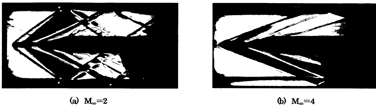
Fig.4 Schlieren photographs of the supersonic flows around a wedge ( semi vertex angle 8.5^\circ )
