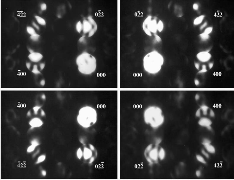
FIG. 3. Dark-field CBED patterns of the  $[0,1,1]$  zone axis at  $T=10$  K for  $\text{PrRu}_4\text{P}_{12}$ . The centers of each disk at  $(0,0,0)$ ,  $(0,2,\bar{2})$ ,  $(4,0,0)$ ,  $(4,2,\bar{2})$  and at counter positions with these reflections are located at exact Bragg positions. Mirror symmetry is observed along the  $(1,0,0)$  plane.
