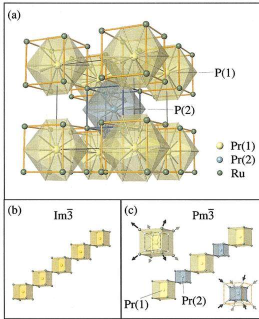
FIG. 4. (Color) (a) Crystal structure of  $\text{PrRu}_4\text{P}_{12}$  in the  $Pm\bar{3}$  phase. (b, c) Schematic diagram of  $\text{PrRu}_8$  cubes in (b)  $Im\bar{3}$  and (c)  $Pm\bar{3}$  phases connected at the corners in the (1,1,1) direction. In the  $Pm\bar{3}$  phase, two kinds of  $\text{PrRu}_8$  cubes are present. The displacement of the Ru atoms in the transition from the  $Im\bar{3}$  to the  $Pm\bar{3}$  phase is depicted in panel (c).
