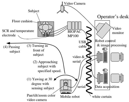
Fig. 1. Top view of experimental setup
