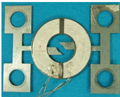
Fig. 1 Ring-type stator vibrator with vibrating pieces.
