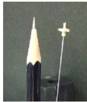
Fig.6 Trial motor using a slender(0.5mm \phi ) ultrasonic transmission line.
