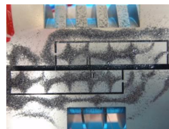
Fig.5 Chladni's sand figure of vibrator.
