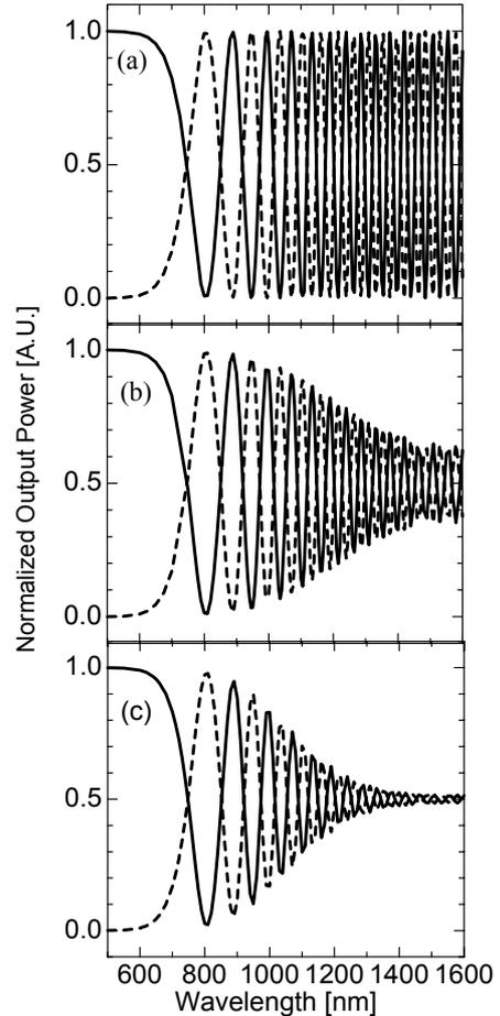
Fig.3 Dependence of power coupling on the wavelength under the conditions of  $C_1=0$ ,  $T_0=100$  fs,  $P_0=10$  kW in (a),  $C_1=-0.2$  ps/m,  $T_0=100$  fs,  $P_0=10$  kW in (b),  $C_1=-0.2$  ps/m,  $T_0=50$  fs,  $P_0=10$  kW in (c) (— Through, - - - - Coupled)
