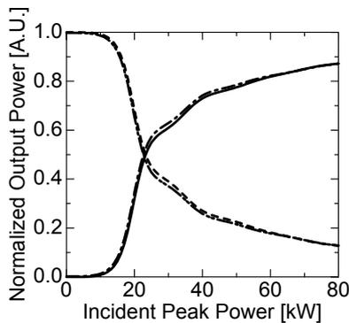
Fig.2 Dependence of power coupling on the incident peak power under the conditions of  $C_1=0$  (— Through, - - - - Coupled) and  $C_1=-0.09$  ps/m (— · — Through, · · · · Coupled)
