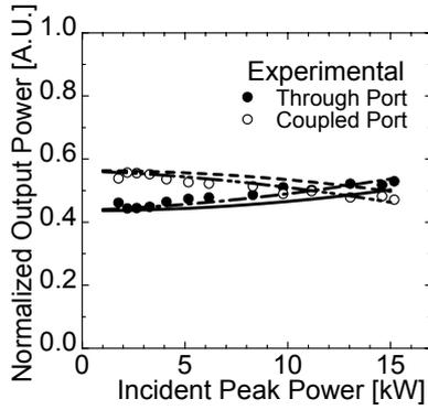
Fig.5 Comparison of experimental power coupling dependent on incident peak power with the numerical results under the conditions of  $C_1=0$  (— Through, - - - - Coupled) and  $C_1=-0.16$  ps/m (- · - · Through, - - - - Coupled)
