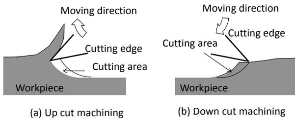
Fig. 10 Cutting situations at maximum cutting force
