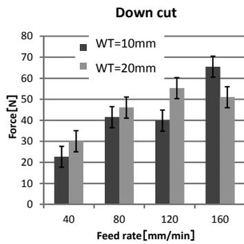
Fig. 5 Cutting force in down cut machining
