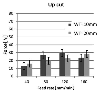
Fig. 4 Cutting force in up cut machining
