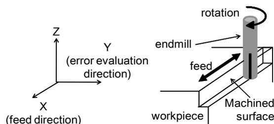
Fig. 1 Side-milling
