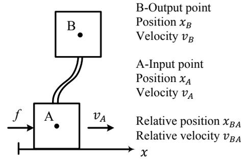
Fig. 1 Rectilinear motion of a flexible structure
