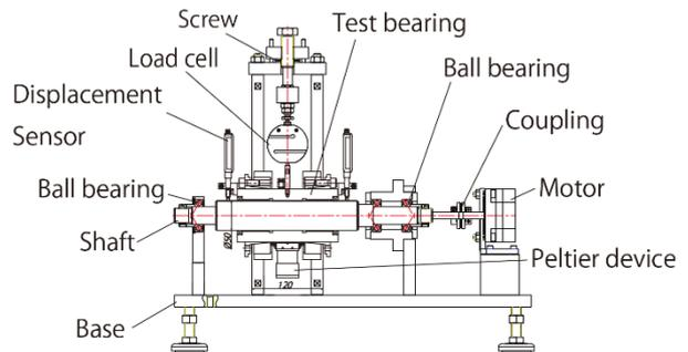
Fig. 1 Test rig of the hydrodynamic journal bearing
