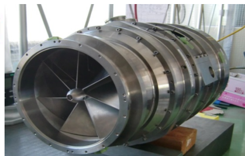
Figure 2 GG-ATR Engine developed in Muroran Institute of Technology
