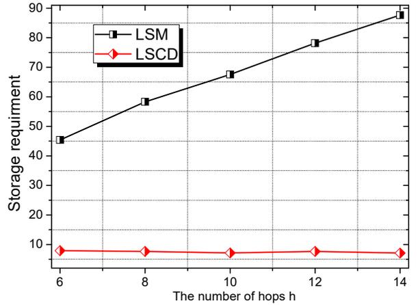
Fig. 9 Storage requirements under different network scales.
