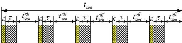
Fig. 4 TDSFK scheme (sensing frequency is  $k$ )
