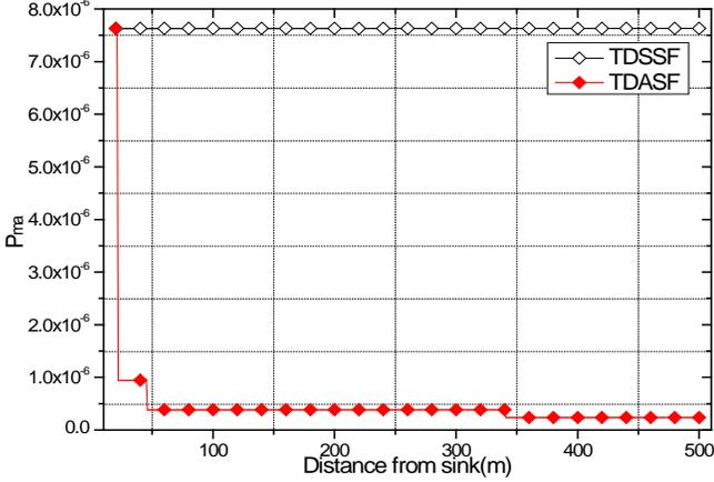
Fig. 10 Probability of missed multiple-target detection ( $P_{ma}$ )
