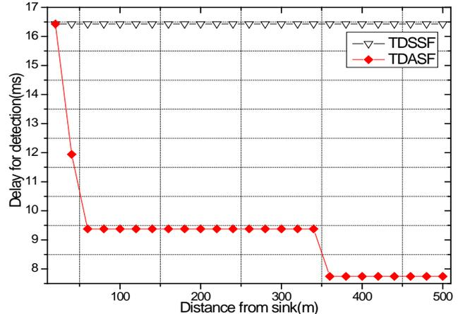
Fig. 12 Detection delays at different distances from sink
