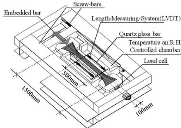
Fig.5 Quasi-fully restraint test (VRTM)<sup>(7)</sup>
