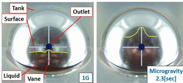
Fig. 6 Liquid behavior in Experiment No. 1.
