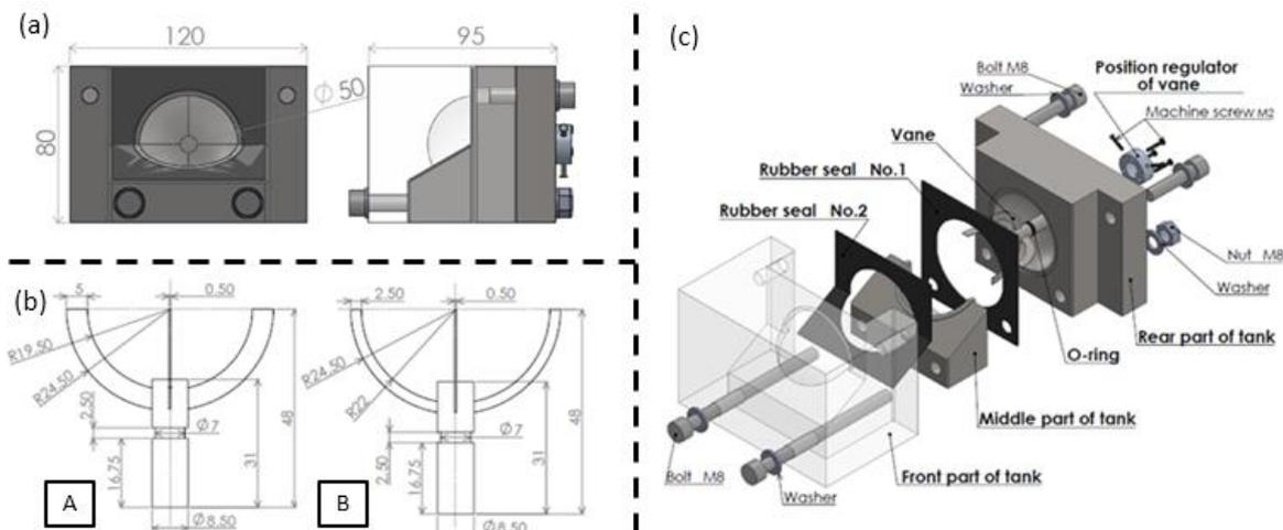
**Fig. 2** Overview of water tank: (a) entire view of water tank, (b) vane configuration, (c) exploded view of water tank.
