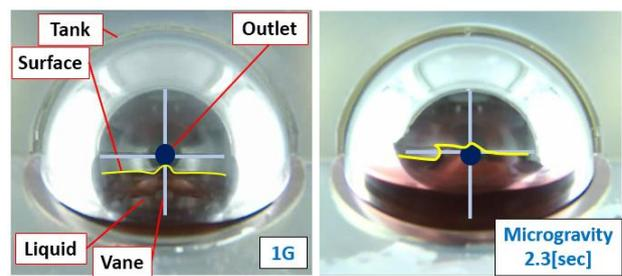
Fig. 7 Liquid behavior in Experiment No. 2.
