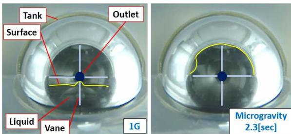
Fig. 8 Liquid behavior in Experiment No. 3.
