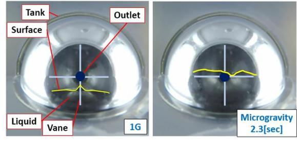
Fig. 9 Liquid behavior in Experiment No. 4.
