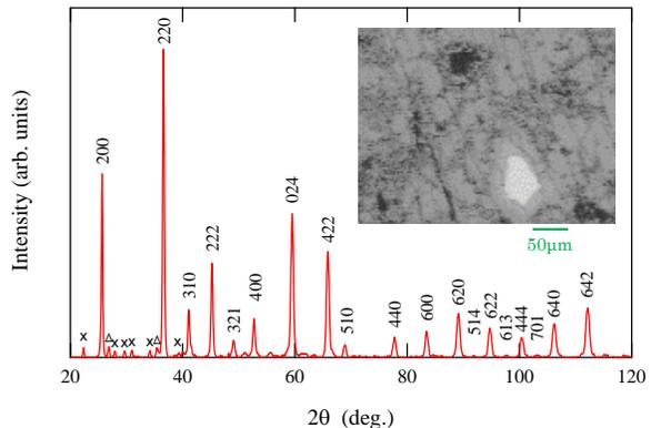
FIG. 1. (Color online) Powder x-ray diffraction results for  $\text{CaOs}_4\text{P}_{12}$ . All the peaks except the tiny peaks due to impurities can be indexed to the cubic ( $\text{Im}\bar{3}$ ) symmetry. Diffraction indexes have been assigned to each peak, which were used to calculate the lattice parameter. The peaks marked by triangles and crosses are attributed to the secondary phases  $\text{OsP}_2$  and  $\text{OsP}_4$ , respectively. The inset shows the electron backscattering SEM image.
