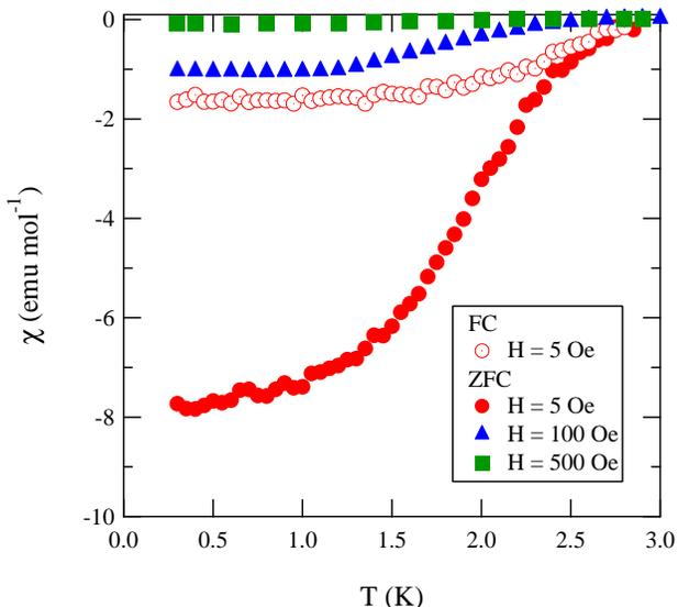
FIG. 4. (Color online) Temperature dependence of the dc magnetic susceptibility of  $\text{CaOs}_4\text{P}_{12}$  below 3 K with 5 Oe (filled circle), 100 Oe (filled triangle), and 500 Oe (filled square) after zero field cooling (ZFC) and with 5 Oe after field cooling (FC; open circle).
