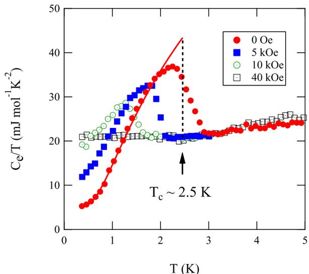
FIG. 5. (Color online) Electronic specific heat contribution  $C_e$  of  $\text{CaOs}_4\text{P}_{12}$  under various fields, plotted as  $C_e/T$  vs  $T$ . The solid line represents the heat capacity based on the model of a spin-singlet fully gapped Bardeen-Cooper-Schrieffer (BCS) superconductor as numerically computed by Mühlischlegel (see text for details).
