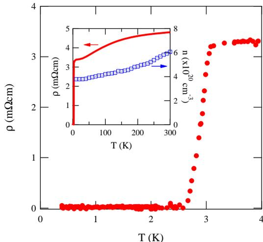
FIG. 2. (Color online) Temperature dependence of the electrical resistivity ( $\rho$ ) below 4 K. The red line for the left axis of the inset shows  $\rho(T)$  up to 300 K. The square symbol for the right axis of the inset shows the carrier concentration  $n$ , up to 300 K.
