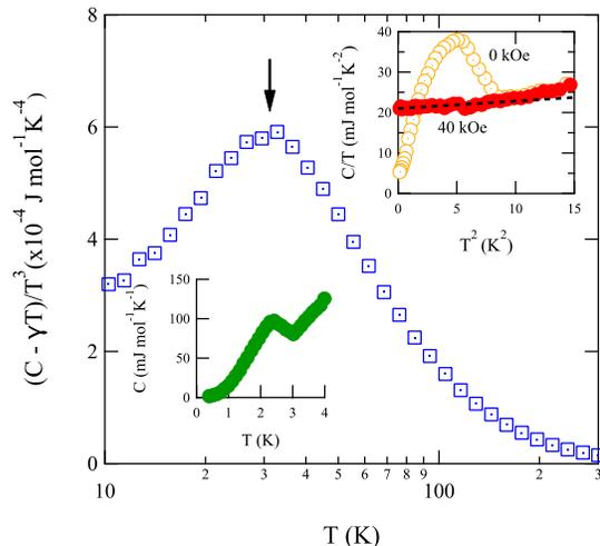
FIG. 3. (Color online) Temperature dependence of the phonon contribution of the specific heat ( $C$ ) plotted as  $(C - \gamma T)/T^3$ . The left-bottom inset shows the temperature dependence of  $C$ . The top-right inset shows  $C/T$  vs.  $T^2$  at zero-field (open circle) and under a field of 40 kOe (filled circle). The dashed line indicates a linear fit.
