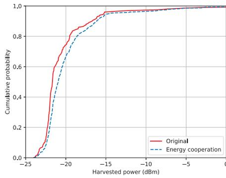
Fig. 5. Cumulative probability of each node harvested power
