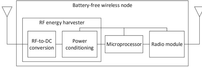
Fig. 1. Battery-free wireless node with RF energy harvesting
