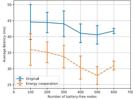
Fig. 10. Average latency with different number of nodes
