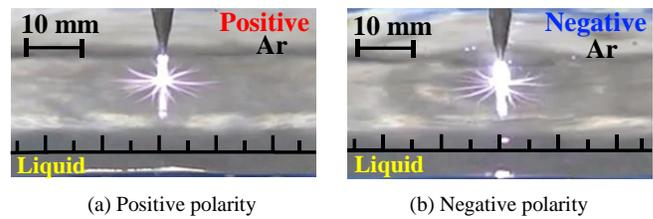
Fig. 2. Photographs of single pulsed discharge propagation.
