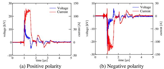
Fig. 3. Waveforms of discharge voltage and discharge current.
