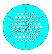
Fig. 1. (Color online) Elliptical-hole core circular-hole holy fiber (EC-CHF).
