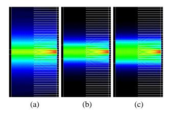
Fig. 9. (Color online) Wave propagation through the interface between a symmetric three-layer slab waveguide and a multilayer planar waveguide with thin air layers. (a)  $a_{\rm SMF}=1\mu{\rm m}$ . (b)  $a_{\rm SMF}=3\mu{\rm m}$ . (c)  $a_{\rm SMF}=5\mu{\rm m}$ .
