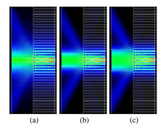
Fig. 8. (Color online) Wave propagation through the interface between a symmetric three-layer slab waveguide with a core layer width of  $a_{\rm SMF}$  and a multi-layer planar waveguide with thick air layers. (a)  $a_{\rm SMF}=1\mu{\rm m}$ . (b)  $a_{\rm SMF}=3\mu{\rm m}$ . (c)  $a_{\rm SMF}=5\mu{\rm m}$ .
