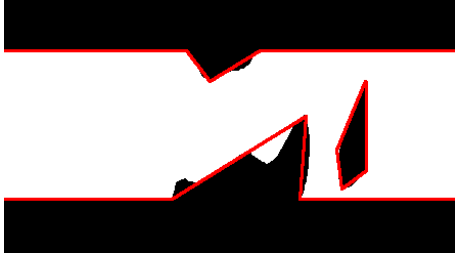
Fig. 2. Topology optimal plasmonic optical diode given in [28]. Black color indicates silver and white means air.
