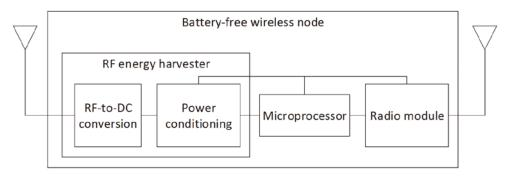
Fig.1 Battery-free wireless node with RF energy harvesting
