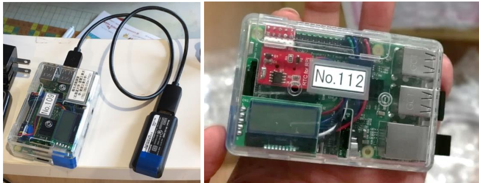
Figure 2.2 The Wi-Fi packet sensing device.
