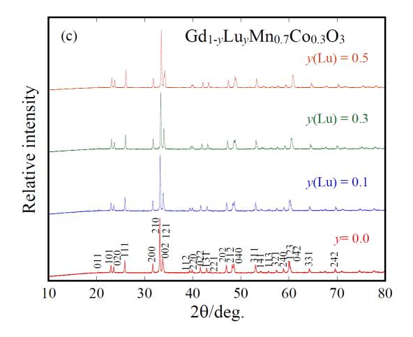
Fig. 1. XRD patterns for  $Gd_{1-y}R_yMn_{0.7}Co_{0.3}O_3$  with y=0.1, 0.3 and 0.5 with substitution by the nonmagnetic elements La, Y and Lu. (a), (b), and (c) correspond to  $Gd_{1-y}La_yMn_{0.7}Co_{0.3}O_3$ ,  $Gd_{1-y}Y_yMn_{0.7}Co_{0.3}O_3$ , and  $Gd_{1-y}Lu_yMn_{0.7}Co_{0.3}O_3$ , respectively,
