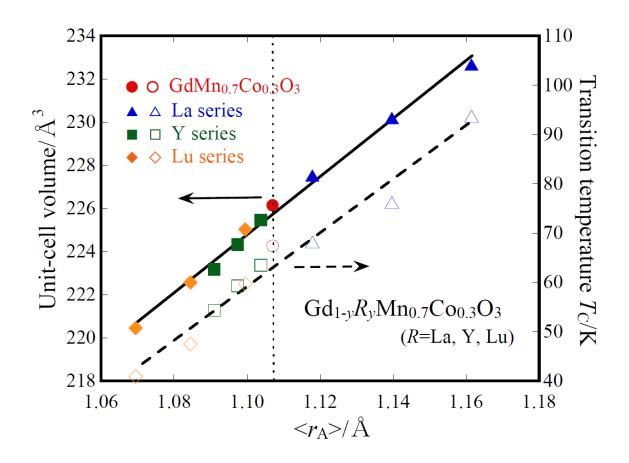
Fig. 4. *V* and  $T_{\rm C}$  as a function of  $\langle r_{\rm A} \rangle$ . Their linear dependence with the same slope suggests that there is a correlation between *V* and  $T_{\rm C}$ . The dotted line denotes the ion radius of Gd<sup>3+</sup>.
