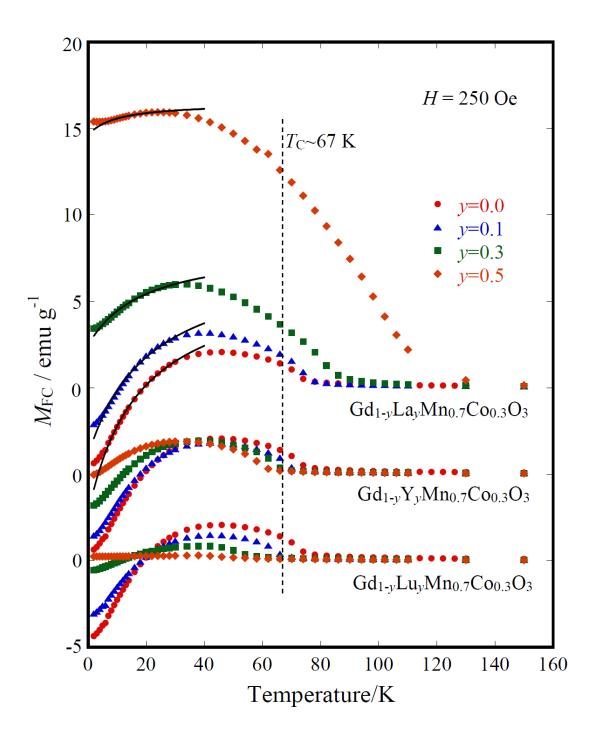
Fig. 3. Temperature dependence of  $M_{FC}$  for  $Gd_{1-y}R_yMn_{0.7}Co_{0.3}O_3$ . Broken line shows  $T_C$  for  $GdMn_{0.7}Co_{0.3}O_3$ . The solid lines in La series are fits using Eq. (4).
