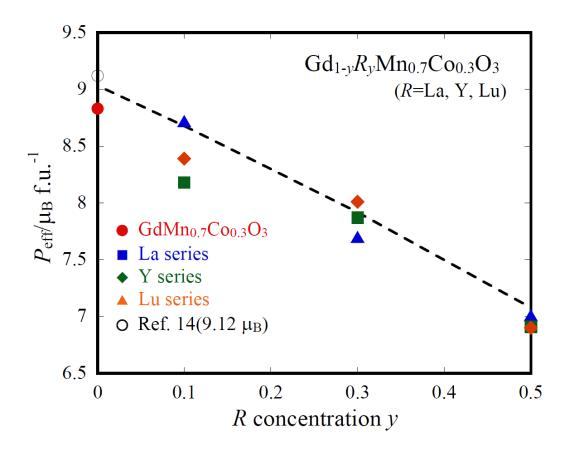
Fig. 6. *R* concentration dependence of effective magnetic moment  $P_{\text{eff}}$  for  $\text{Gd}_{1-y}R_y\text{Mn}_{0.7}\text{Co}_{0.3}\text{O}_3$  (*R*=La, Y, and Lu).
